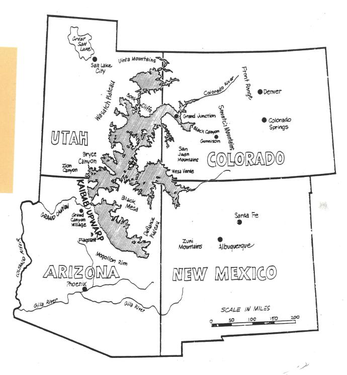
A computer was asked to draw the shoreline of the lake which would form behind the Kaibab Upwarp if the Grand Canyon were blocked at the 5,700-foot elevation. The lake which would form is shown above. It would contain the water of three Great Lakes. This computer-generated lake approximates the outline of the ancient lake which breached its dam to form Grand Canyon.
